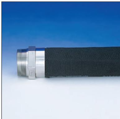
Woven from thousands of nylon filaments into an abrasion-resistant sleeve, the nylon cover extends individual hose life in severe abrasive environments. As it is scuffed and worn, its filaments frizz, forming an even thicker, more protective shield.
